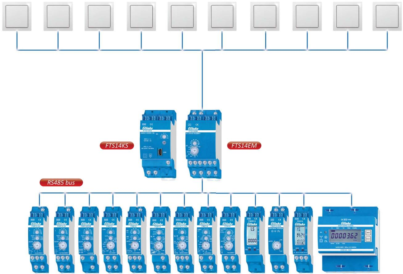
All optional possibilities can be combined as required: FTS14EM with actuators, the wireless antenna module FAM14, the pushbutton wireless output module FTS14FA and the pushbutton gateway FTS14TG for connection to pushbutton couplers FTS61BTK.
