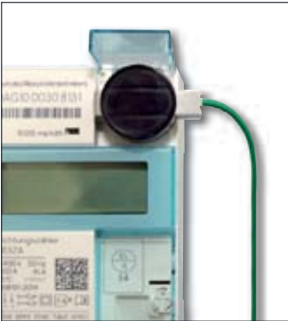
IR scanner for energy meters
