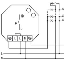
4-wire circuit with attic lighting, resettable.
