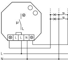
3-wire circuit, resettable.
