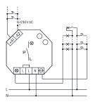
4-wire circuit with attic lighting, resettable
