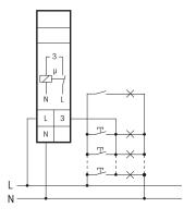
3-wire circuit with attic lighting, not resettable.
