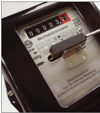
Scanner for Ferraris meter AFZ
