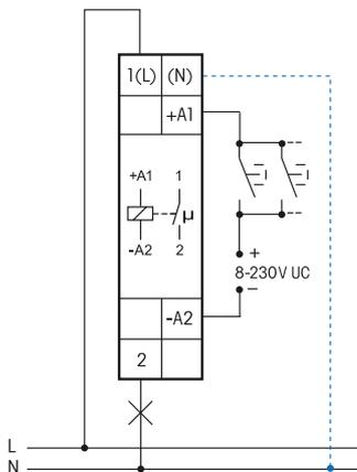
If N is connected, the zero passage switching is active.
