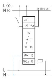
If N is connected, the zero passage switching is active.
