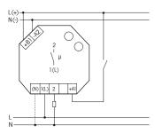
If N is connected, the zero passage switching is active.
