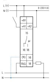
If N is connected, the zero passage switching is active.
