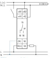
If N is connected, the zero passage switching is active.
