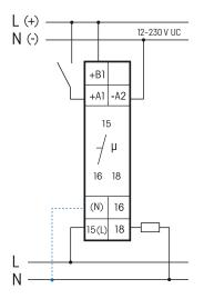
If N is connected, the zero passage switching is active.
