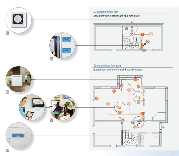
For the one-family house we recommend the mounting of the wireless actuators in a distribution cabinet or sub-distributor per floor.
