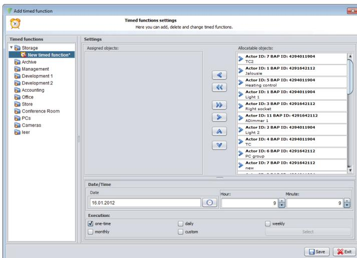
4. In the right list all existing FVS actuators, connections and system functions are listed.
