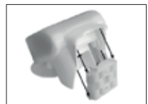
Fig. 11 Push the housing from above into the fastened mount. The bumps on the mount must snap into the rails in the housing.
