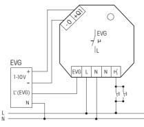
For the control from several LED drivers with 1-10V passive interface, an additional voltage source is necessary, this can be the power supply unit SNT12-230V/12V DC-0.5A or SNT61-230V/12V DC-0.5A, in both cases a 1k0hm resistor is necessary.
