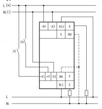
When the (N) is connected, the contact switching is active in the zero crossing.
