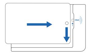
The OnWall has a sliding Lightning charging connector that can be moved by hand and thus adapted to the size of the iPad.
