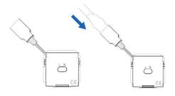
2. Plug the OnWall's USB ribbon cable into the USB-A socket on the power supply unit.
