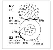
With the lower rotary switch on the front two operate voltages resp. dropout voltages can be set and the number of monitored phase conductors must be selected.
