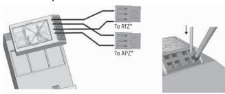
Remove the fuse cover on the MUA-100. Insert the SM/MUA-100 fuse module (article number: 28380004) from above and press down until it clicks into place. To insert the control cables to the APZ and RfZ into the terminals, open the terminals with a screwdriver.
