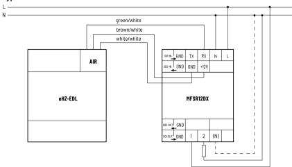
If (N) is connected, the zero passage switching is active.
