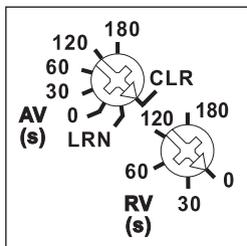
The upper rotary switch **AV** is required for teach-in. Then set here the response lag time AV between 0 and 180 seconds for Contact L-2.
