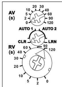
**Use the top rotary switch AV** to set the response lag time AV between 0 and 120 seconds for Contact L-1.
