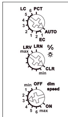
**The upper rotary switch** determines the operation, whether automatic lamp detection or special comfort positions should work:
