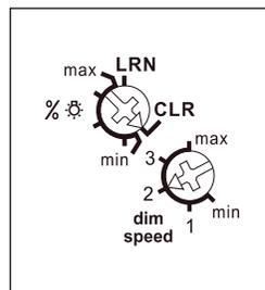
**The minimum brightness (fully dimmed) is adjustable with the % rotary switch.**
