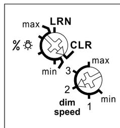
**The minimum brightness (fully dimmed) is adjustable with the %&#x2602; rotary switch.** In the setting LRN up to 35 wireless pushbuttons can be assigned therefrom one or more central pushbuttons.
