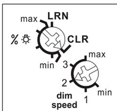
**The minimum brightness (fully dimmed) is adjustable with the % rotary switch.** In the setting LRN up to 35 wireless pushbuttons can be assigned therefrom one or more central pushbuttons.
