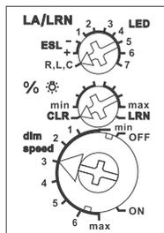
The top rotary switch LA/LRN is first required for teach-in and in operation, it defines what load type the dimming curve should be set to: **Position R, L, C** is the setting for all load types except for ESL and LED. In particular for 230V glow and halogen lamps. The load type, inductive or capacitive, is detected automatically.
