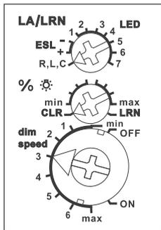
The top rotary switch LA/LRN is first required for teach-in and in operation, it defines what load type the dimming curve should be set to:
