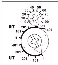
The lower rotary switch defines the group to which an FTS14EM belongs. A total of 5 groups are available (1, 101, 201, 301 and 401) each with 100 IDs. The upper rotary switch (0 to 90) sets the ID within a group. The ID range within a group results from the combination of upper and lower rotary switches and must be set differently on each FTS14EM. Maximum ten FTS14EMs form a group. Therefore, a total of 500 FTS14EMs comprising 500 pushbuttons or contacts are possible in one RS485 bus.
