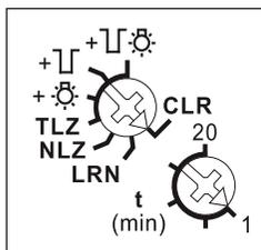
**With the top rotary switch** in the setting LRN up to 35 wireless pushbuttons and/or wireless motion/brightness sensors FBH can be assigned of which one or more central pushbuttons. The required function of this staircase off-delay timer can then be selected.
