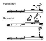
Note: when changing the battery, the mode (operating mode) is retained. Mode 1 is pre-set on delivery.
