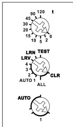
**Use the rotary switches** to teach-in the pushbuttons and test the device as required. For normal mode, the middle and lower rotary switches are then set to AUTO. With the upper rotary switch the EW time (0-120 seconds) is directly set for relays or the RV time (0-120 minutes) for impulse switches for all channels if necessary.
