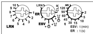
**With the middle rotary switch on the side** in the setting LRN up to 35 wireless pushbuttons can be assigned, of which one or more central control pushbuttons. In addition wireless window/door contacts with the function N/O contact or N/C contact while the window is open. The required function of the impulse switch with integrated relay function can then be selected:
