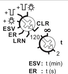
**With the top rotary switch** in the setting LRN up to 35 wireless pushbuttons can be assigned therefrom one ore more central control pushbuttons. In addition wireless window/door contacts with the function N/O contact or N/C contact while the window is open. The required function of the impulse switch with integrated relay function can then be selected:
