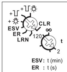
With the top rotary switch in the setting LRN up to 35 wireless pushbuttons can be assigned therefrom one or more central control pushbuttons. In addition wireless window/door contacts with the function N/O contact or N/C contact while the window is open. The required function of the impulse switch with integrated relay function can then be selected:
