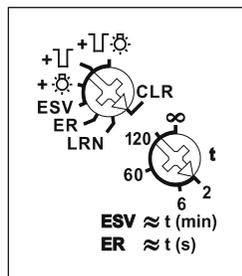
With the **top rotary switch** in the setting LRN up to 35 wireless pushbuttons can be assigned therefrom one or more central control pushbuttons. In addition wireless window/door contacts with the function N/O contact or N/C contact while the window is open, wireless outdoor brightness sensors FAH and wireless motion/brightness sensors FBH. The required function of the impulse switch with integrated relay function can then be selected:
