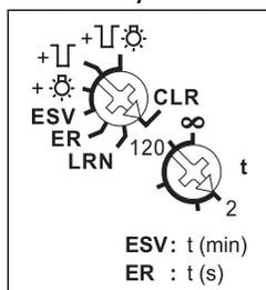
With the top rotary switch in the setting LRN up to 35 wireless pushbuttons can be assigned therefrom one or more central control push-buttons. The required function of the impulse switch with integrated relay function can then be selected:
