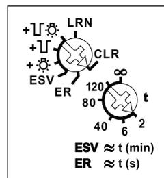
**With the top rotary switch** in the setting LRN up to 35 wireless pushbuttons can be assigned, of which one or more central control pushbuttons. In addition wireless window/door contacts with the function N/O contact or N/C contact while the window is open. The required function of the impulse switch with integrated relay function can then be selected:
