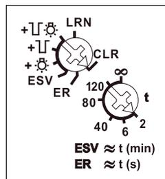
**With the top rotary switch** in the setting LRN up to 35 wireless pushbuttons can be assigned therefrom one ore more central control pushbuttons. In addition wireless window/door contacts with the function N/O contact or N/C contact while the window is open, wireless outdoor brightness sensors FAH and wireless motion/brightness sensors FBH. The required function of the impulse switch with integrated relay function can then be selected:
