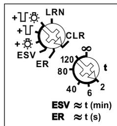
**With the upper rotary switch** in the setting LRN up to 35 wireless pushbuttons can be assigned therefrom one or more central control pushbuttons. In addition wireless window/door contacts with the function NO contact or NC contact while the window is open, wireless brightness sensors and wireless motion/brightness sensors. The required function of the impulse switch with integrated relay function can then be selected:
