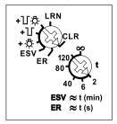
With the upper rotary switch in the setting LRN up to 35 wireless pushbuttons can be assigned therefrom one ore more central control pushbuttons. In addition wireless window/door contacts with the function NO contact or NC contact while the window is open, wireless brightness sensors and wireless motion/brightness sensors. The required function of the impulse switch with integrated relay function can then be selected:
