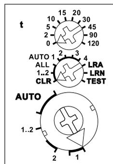
**Use the rotary switches** to teach-in the buttons and test the 4 channels as required. For normal mode, the middle and lower rotary switches are then set to AUTO. With the upper rotary switch the EW time (0-120 seconds) is directly set for relays or the RV time (0-120 minutes) for impulse switches for all channels if necessary.
