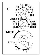
**Use the rotary switches** to teach-in the buttons and test the 2 channels as required. For normal mode, the middle and lower rotary switches are then set to AUTO. With the upper rotary switch the EW time (0-120 seconds) is directly set for relays or the RV time (0-120 minutes) for impulse switches for all channels if necessary.
