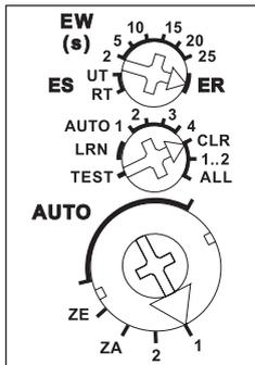
The upper rotary switch defines the function of the 2 channels together as impulse switch with universal switch (ES-UT), as impulse switch with direction switch (ES-RT), as fleeting NO contact (EW) or as relay (ER).
