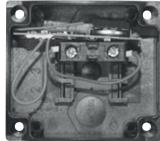
EATON M22-D-G-X1/KC11/I: The 2 red wires are provided with ferrules and connected to the 'green' button NO.
