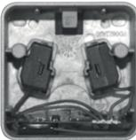
NICE EKSEU: The 2 red wires are connected to the left button, the 2 blue wires to the right button, each to terminals 0 and NO.
