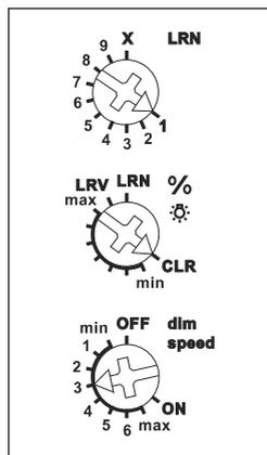
If the upper rotary switch is set to X, special functions are active, which must be settled with the PC Tool PCT14.
