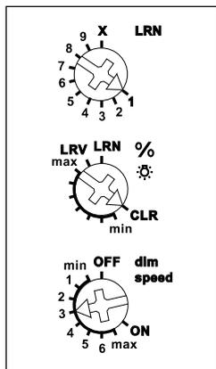
The minimum brightness (fully dimmed) is adjustable **with the % rotary switch**.
