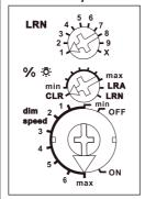
If the upper rotary switch is set to X, special functions are active, which must be settled with the PC Tool PCT14.
