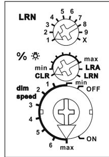
The minimum brightness (fully dimmed) is adjustable **with the % rotary switch**. The dimming speed is adjustable using the **dimming speed rotary switch**.
