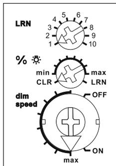
The minimum brightness (fully dimmed) is adjustable with the % CLR rotary switch. In the setting LRN up to 35 wireless pushbuttons can be assigned therefrom one or more central pushbuttons.
