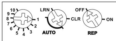
The left rotary switch on the side is required to teach-in the direction button if required.
