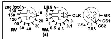
With the middle rotary switch on the side in the setting LRN up to 35 wireless pushbuttons can be assigned, of which one or more central pushbuttons. Then the automatic turning system (WA) is set using the same rotary switch.
